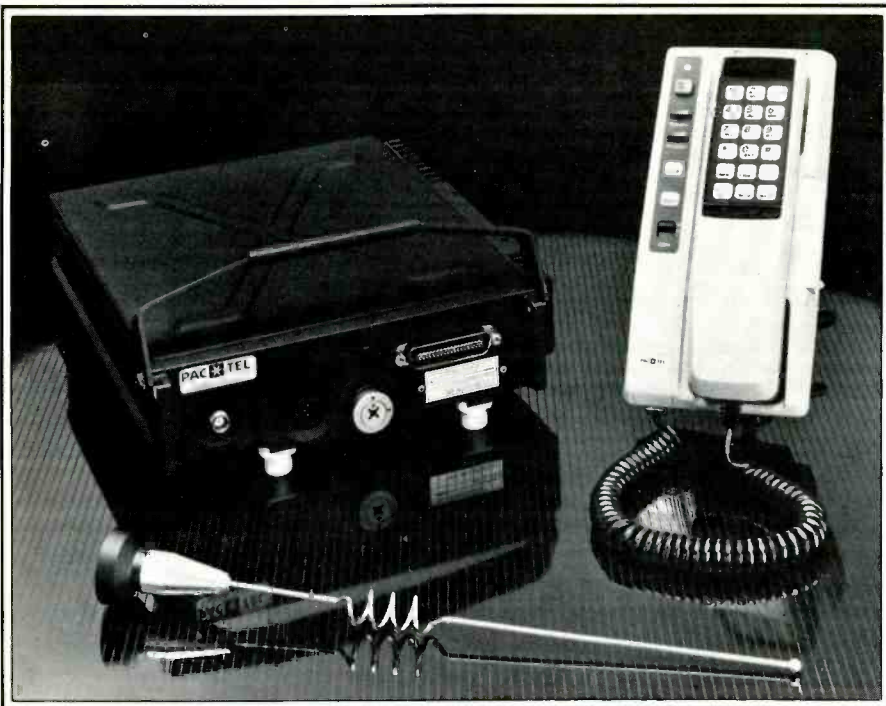
A mobile cellular system consists of three major components: the remote control head with handset, the trunk-mounted transceiver, and the antenna.
